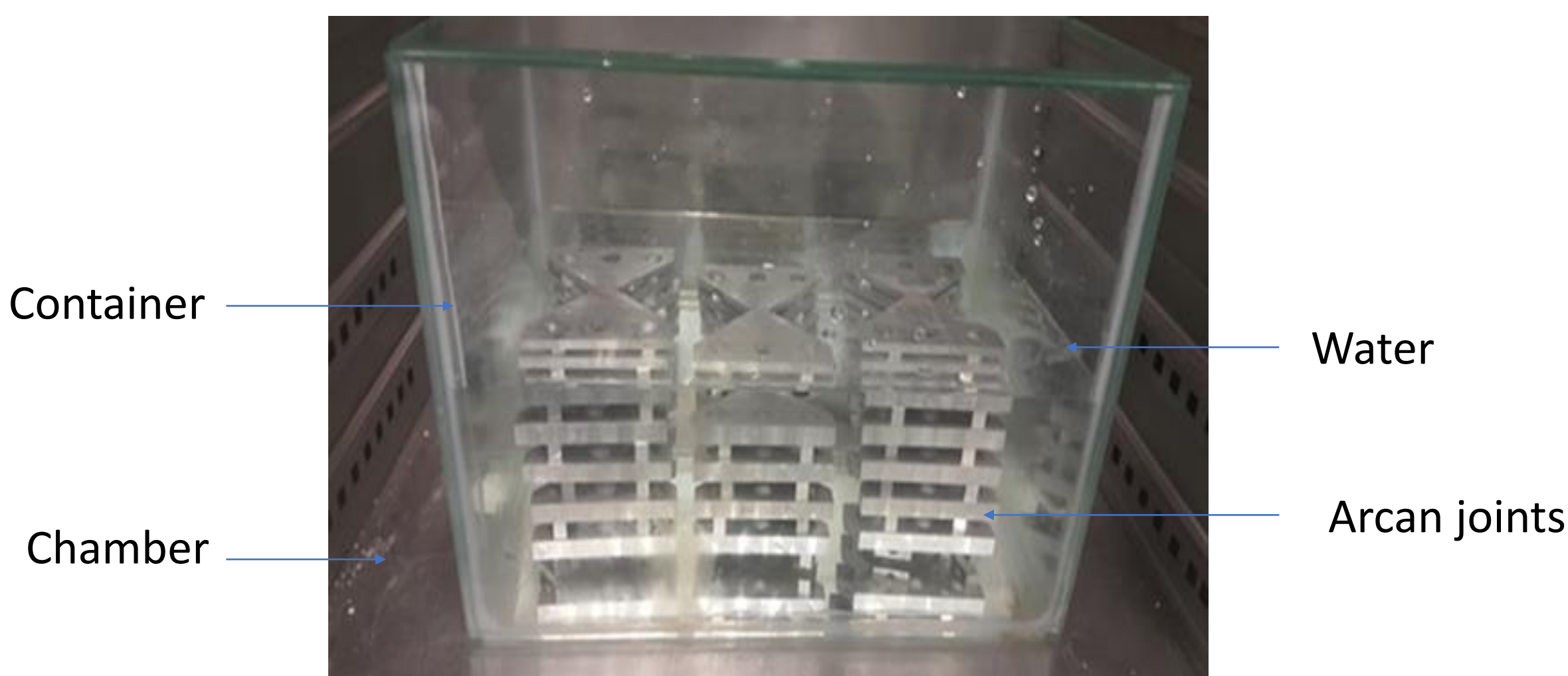
Figure 3 – Ageing of Arcan joints
